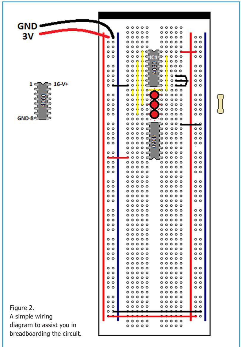
Figure 2. A simple wiring diagram to assist you in breadboarding the circuit.
